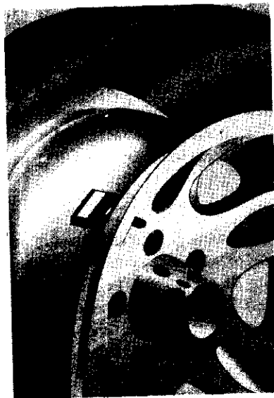
Figure 13-5 Wireless sensor application—tire pressure sensing (Courtesy of Schrader Electronics).
